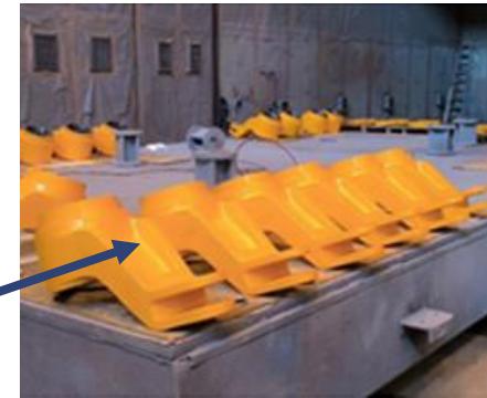
Wicket gates & WG levers
