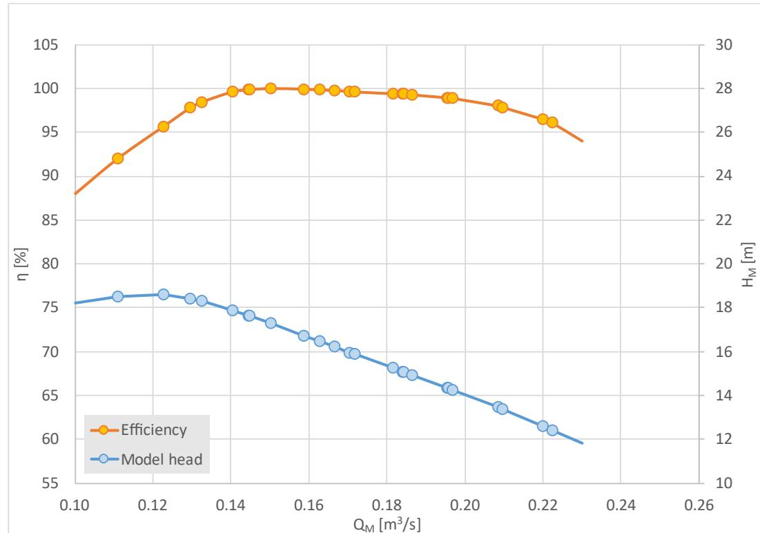
Target Pump mode performance curve
