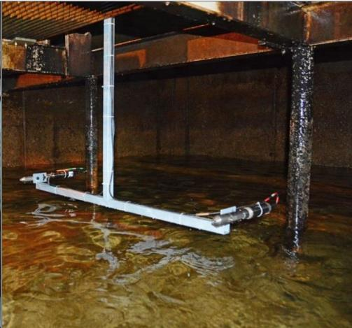
Tailwater measurement section
